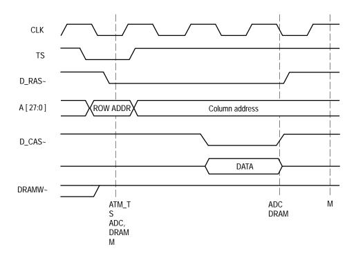
Figure 2-3: Byte Read transfer in normal mode with 8-bit EDO Dram
