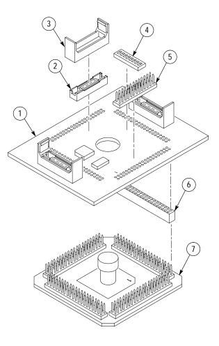
Figure 6–1: MCF5206 probe adapter exploded view
