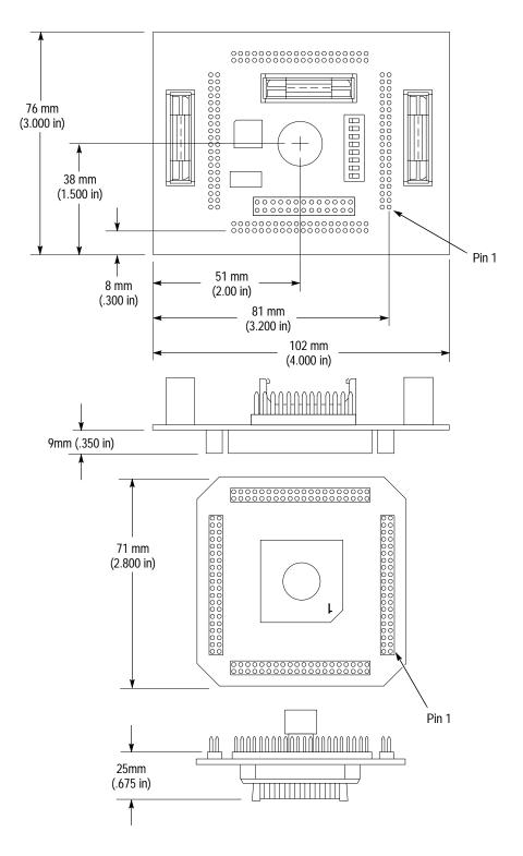
Figure 3–1: Dimensions of the probe adapter
