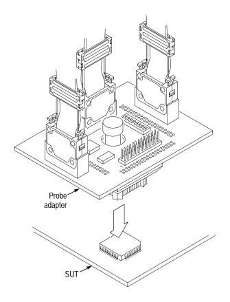
Figure 1-3: Placing the probe adapter onto the SUT
